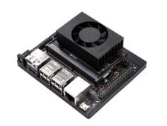
Jetson Nano GPU: 128-core Maxwell CPU: Quad-core ARM A57 Memory: 4 GB
